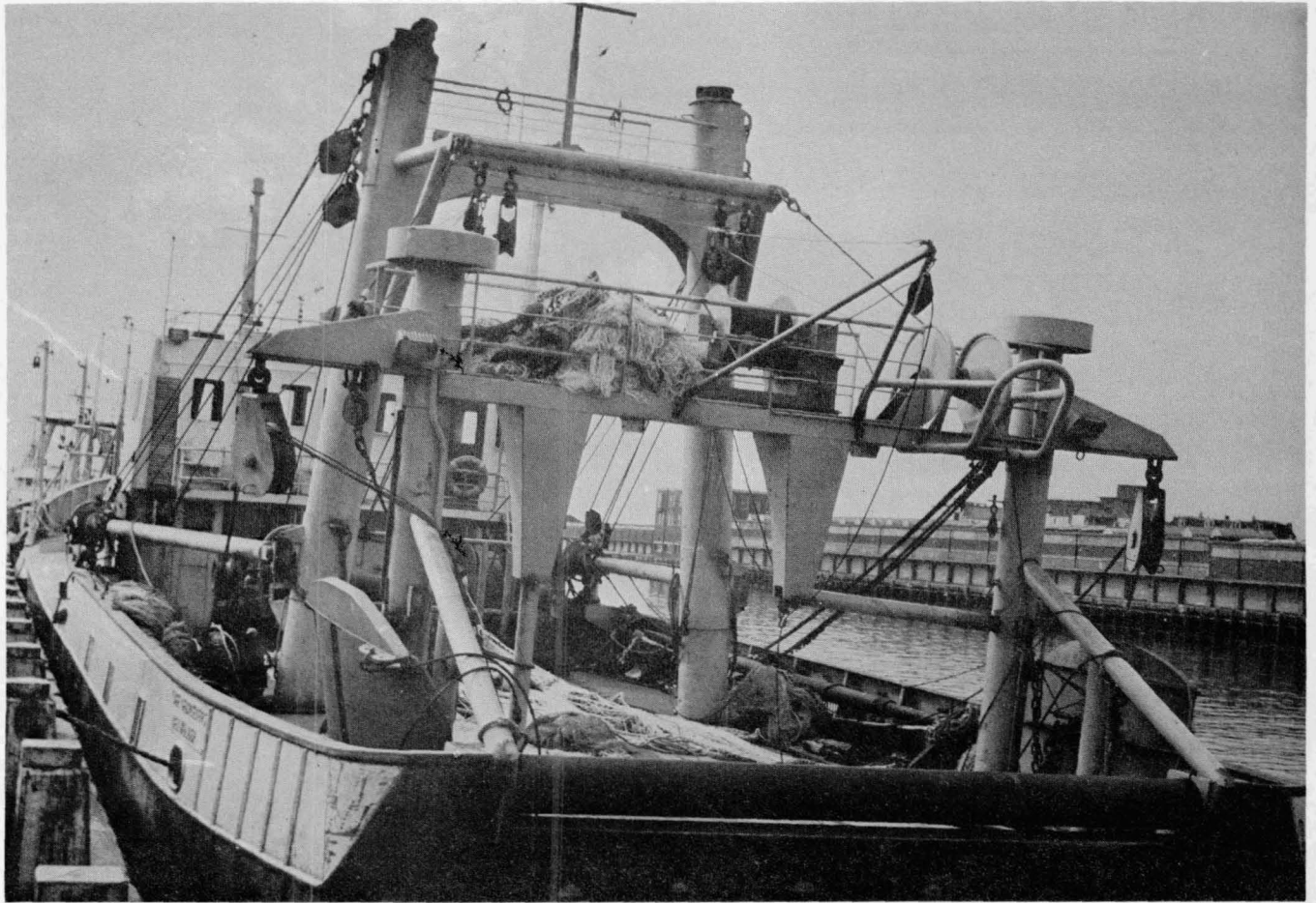
Atdeck of 2000 hp multi-purpose combination wet fish/ freezer stern trawler (L.o.a. 40,5 m)
